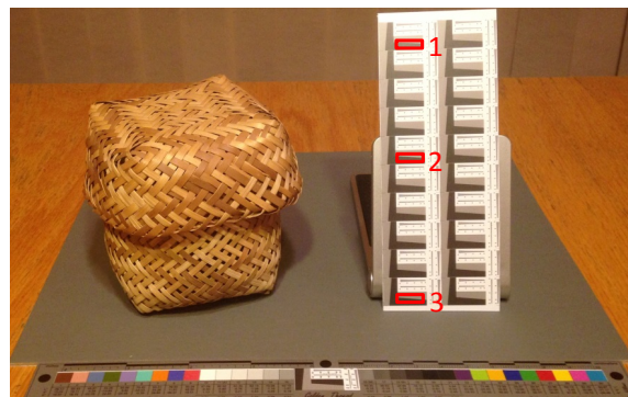
Figure 1: Example image capture setup with two test charts
