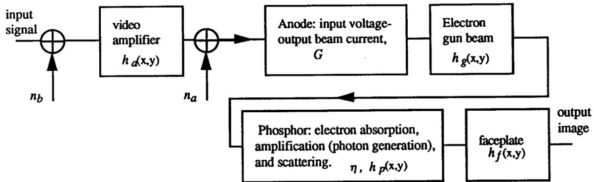
Figure 3. Diagram of CRT imaging model.
