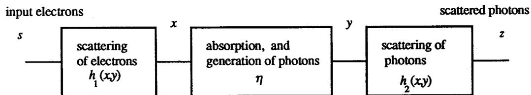
Figure 2. Simple stochastic scattering and absorption model.
