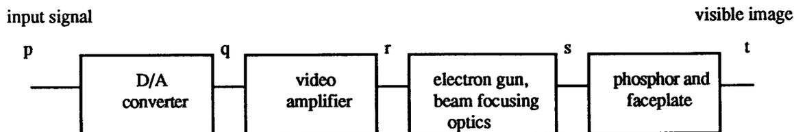
Figure 1. Functional diagram for the CRT model.
